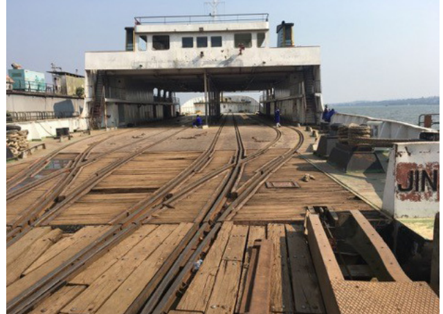
Roll-on / roll-off ferry with railway tracks
